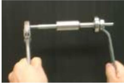
Action (18) : Attach spindle , disc , valve , spring washer , a set of hexagon nuts and spring . Secure bottom cover with 6 hexagon head bolts . **(Tightening torque: 20 N·m)**
