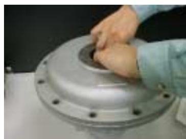
Action (11) : While securely holding top diaphragm plate ②① with hand, unscrew 3 hexagon socket head cap bolts ②⑥.
