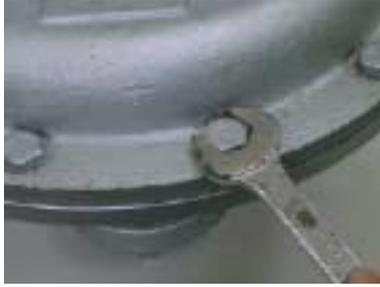
**Presumable cause III.19: Hexagon socket head cap bolt ㉑ and locknut ㉒ are loosened.**
