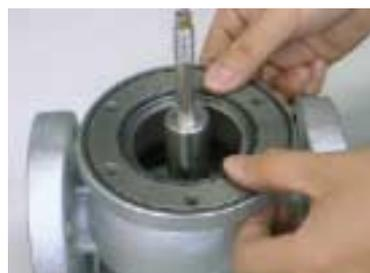
Action (46): Place the bottom diaphragm case and secure it with hexagon socket head cap bolt .
