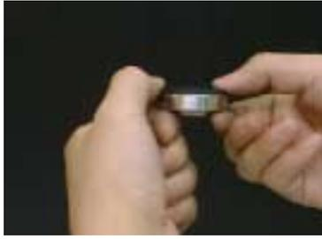
Action (17) : Attach disc , valve , spring washer into spindle and secure with hexagon nut . **(Tightening torque:16 N·m)**
