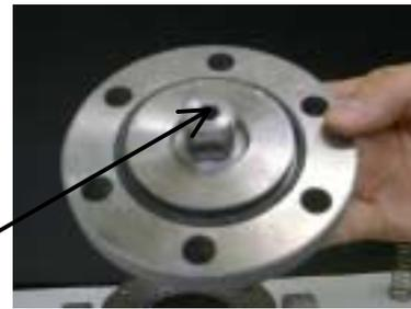
Action (14) : Check disc and valve seat for pinched foreign materials and damage. Remove pinched materials, if any.
