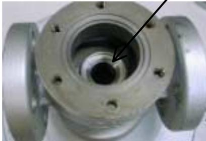
Action (15) : If the valve seat is damaged, consult us. If disc is damaged, loosen hexagon nut and remove spring washer and valve . Remove the disc from recess on the valve .
