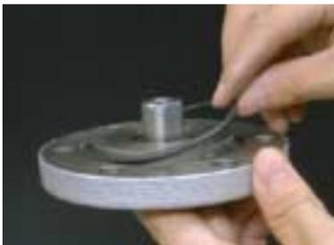
Action (40): Attach the bottom cover and secure it with hexagon head bolt .
