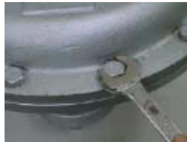
Action (22) : Attach spring ㉙ and spring plate ㉚. Secure spring chamber ㉛ with 6 hexagon head bolts ㉜.
