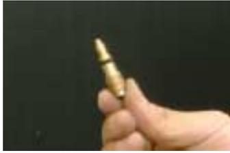
Action (6) : Turn the needle valve to full close and then open by turning one turn in reverse direction with a flat head screwdriver.
