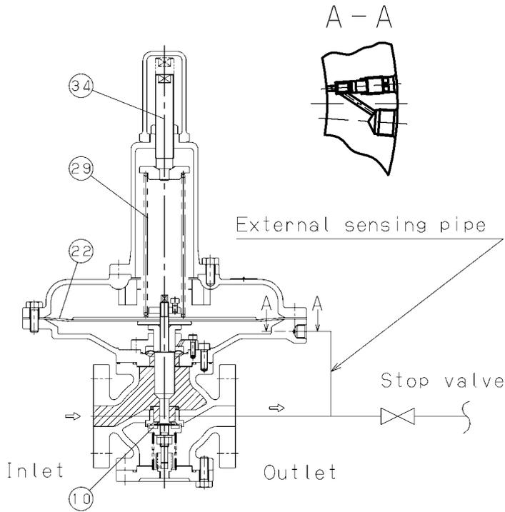
The adjusting screw ③④ compresses the adjusting spring ②⑨ to press down the diaphragm ②③ that will open the directly connected disc .
