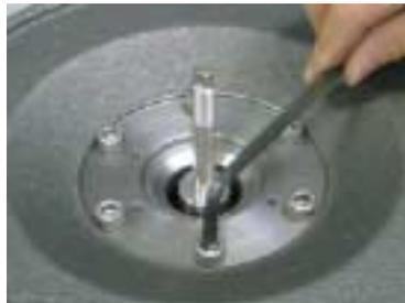
Action (45) : In the case O-ring is damaged, follow steps described in Actions (7) to (12). Unscrew hexagon head bolt ㉔. Remove the bottom diaphragm case and replace the O-ring.
