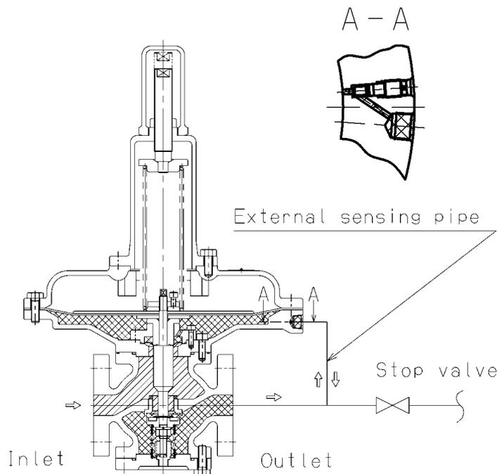
Gradually opening the outlet stop valve proportionally decreases the pressure applied on the diaphragm ②③ until the load from the spring ②⑨ enables the disc to open.
