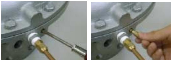
Action (5) : Clean the needle valve and hole of lower diaphragm casing.
